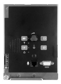
On power-up, the control panel selects Channel 1. During normal operation, pressing 'I' selects Channel 1 and pressing 'II' selects Channel 2. Pressing a channel select button when that particular channel has already been selected has no effect.
